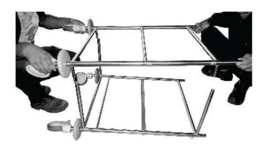
5. Place the bottom tray, lock the skeleton with the brown powder-coated flats and fix the main handle
